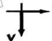
Figure 20.12 (c): Phasor diagram for capacitor.
